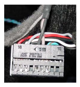
Tip: to open the plugs, stick a small flathead screwdriver in the latch, hold the plug cover with one hand and pull the wires with the other hand:
