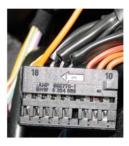
Insert the coaxial (video) wire into cavity #13 (clear) and #14 (black) on the BLUE plug that came with the car's harness
