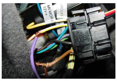
Insert the orange wire into cavity #17 on the WHITE plug
