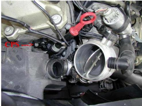
2. Remove the air intake silencer with a 10mm nut-driver:
