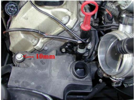
3. Unscrew the 5mm Hex (Allen) Key that holds the CPS in place. Remove the engine cover and disconnect the electrical connector that goes from the CPS to the top of the engine. Yes, the connector end can and will slide behind the oil dipstick, but just barely:
