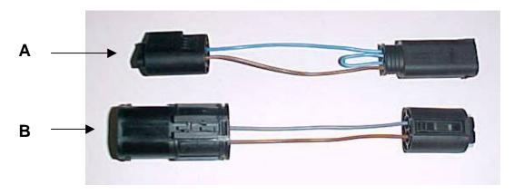
Beginning with harness "A", cut the brown wire at the middle. Cut the <u>looped</u> blue wire flush with the plug where it connects to the plug closest to the brown wire. Strip 1/4" insulation from the hree loose ends.
