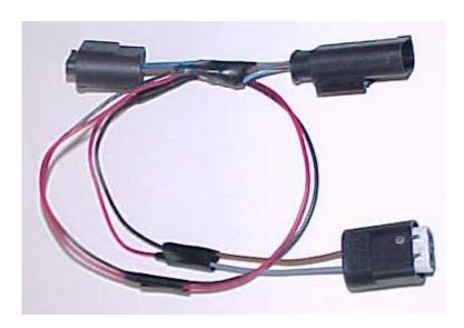
When you're finished, wrap the completed harness in electrical tape (or convoluted tubing like the one below) to give it that "done at the factory" look.
