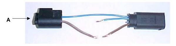
Moving to harness "B" cut both wires flush with the <u>large</u> plug. Trash the large plug & strip 1/4" insulation from the two ends of both wires.
