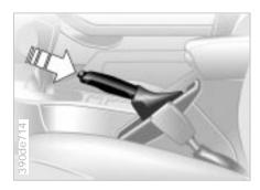
The parking brake is primarily designed to prevent the vehicle from rolling while parked. It operates on the rear wheels.
