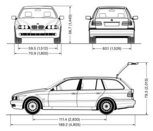
All dimensions are given in inches (mm). Height with roof-mouted luggage rack\*: 57.4 (1,459) Min. turning circle dia.: BMW 525i: 37.1 ft (11.3 m); BMW 540i: 37.4 ft (11.4 m)
