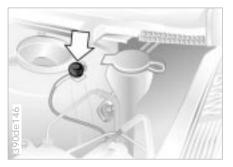
6. Next, connect one end of the other jumper cable (-) to either the support vehicle's negative battery terminal or a suitable ground on its engine or bodywork. Connect the other end to the negative battery terminal or a suitable ground on the vehicle being started. There is a special nut on the strut dome of your BMW; refer to the arrow in the illustration
