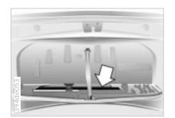
The hazard warning triangle is readily available, stored in the onboard tool kit mounted on the inside of the luggage compartment lid/tailgate.
