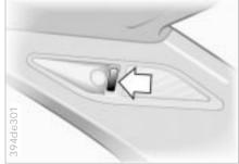
The reading lamps are located in the front near the interior lamp. There are also reading lamps in the rear. They can be switched on and off with the switch (arrow) adjacent to each lamp.
