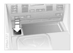
Press the cover panel for access (arrow), then push the lighter down. You can remove the lighter from its socket for use as soon as it snaps back out.
