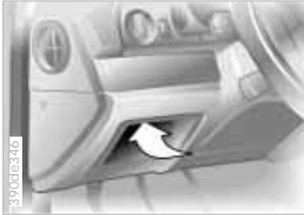
Access to the interface socket for the On-Board-Diagnostics (OBD): lift the cover (arrow) next to the steering column.
