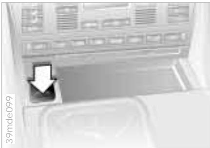
Press the cover panel for access (arrow), then push the lighter down.
