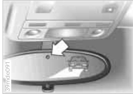
The interior and exterior mirrors with automatic dimming feature reduce the glare from following traffic by adapting the intensity of the reflected images to correspond to levels of light registered by the unit's sensors. The mirrors revert to their undimmed setting as soon as the light source disappears.
