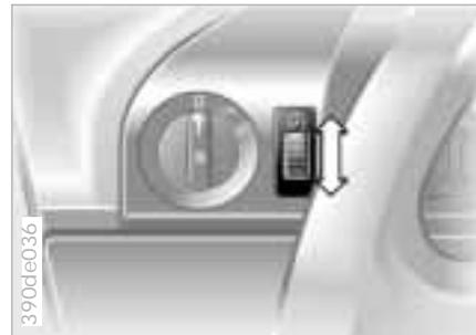
Turn the rotary dial to adjust the lighting intensity.
