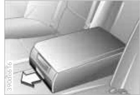
Two beverage holders are provided in the lower section of the center armrest. Pull the handle outward to open (arrow).
