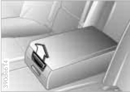
Fold the armrest out and open the cover by lifting the handle (arrow).
