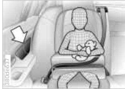
This is the right way for a child to sit in a child restraint when rear side airbags (arrow) are provided.
