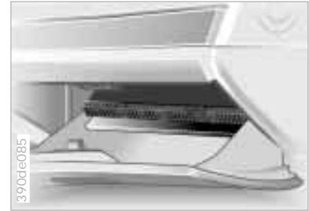
If an electrical accessory should fail, switch it off and check the fuse.
