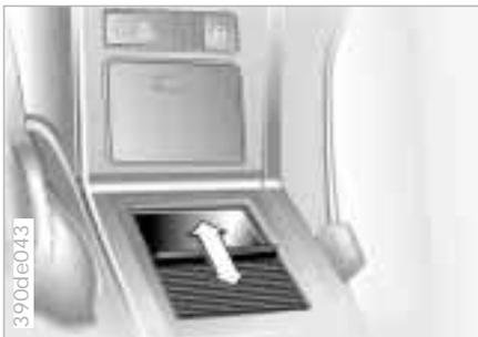
The cover of the storage compartment on the inclined surface of the center console can be pushed open or closed (arrow). If your vehicle is equipped with a cassette holder\*, open each cassette compartment by pressing the small button.
