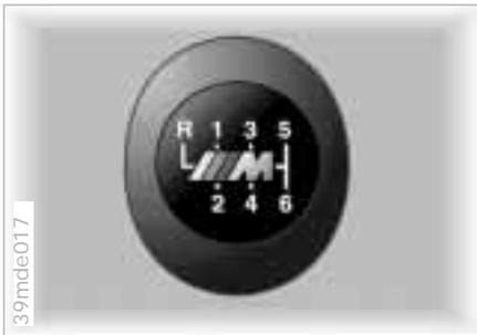
Every time you shift gears, always depress the clutch pedal all the way down, pushing the manual-shift gear lever into the desired position.
