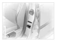
The inflation pressures are indicated on a sticker attached to the B-pillar behind the driver's door (visible with door open).
