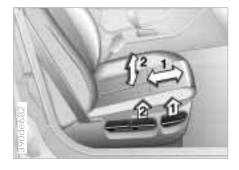
1 Forward/backward adjustment Pull the lever and slide the seat to the desired position.
