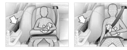
This is the right way for a child to sit in a child restraint when rear side airbags (arrow) are provided.
