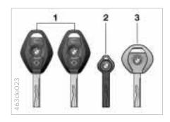
1 The master keys with remote control determine the functions of the Key Memory. Refer to page 60.
