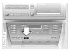
To operate, press the key briefly with the ignition key in position 1 or 2.
