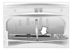
The hazard warning triangle is quickly available, stored in the onboard tool kit mounted on the inside of the luggage compartment lid/tailgate.
