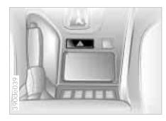
The button flashes rhythmically when the hazard warning flashers are on.
