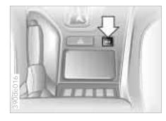
You can operate the central locking system with this button when the driver's door is closed. With this button, only the doors, the luggage compartment lid/tailgate and rear window are unlocked or locked. The anti-theft system is not activated. Also, the fuel filler door remains unlocked to allow refueling.
