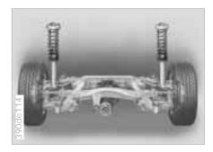
The control arms on the patented integrated aluminum rear axle assembly are not mounted directly on the body. They are mounted elastically on a chassis sub-frame which is joined in turn with elasticity to the vehicle body. The resulting double elastic suspension system effectively absorbs the forces resulting from bumps and road surface irregularities.
