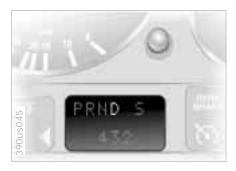
The automatic transmission of your BMW is equipped with Adaptive Transmission Control (ATC), a system which reacts with precision to your individual driving style and the driving conditions. To achieve this, different driving programs are automatically engaged.
