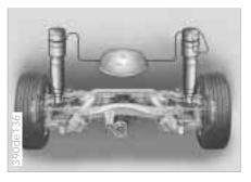
The level control system for the rear axle maintains constant ground clearance of your vehicle, even when carrying a load.
