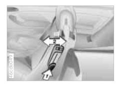
The seat-integrated safety belt system ensures easier access to the back seat. It is not necessary to adjust anything on the safety belt system. It automatically adjusts to different body sizes.
