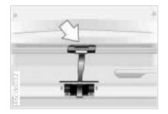
3 Lift the floor panel up with the device designed to hold it and hook it onto the rubber seal of the water gutter (arrow).
