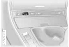
3 Press the button to unlock the top. The lid locks for the convertible top are unlocked and the side windows lower slightly
