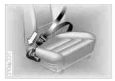
The safety belt tensioners respond to severe head-on collisions by tightening the belts to ensure that occupants remain firmly positioned in their seats. A gas-pressure system retracts the buckle assembly to tension the shoulder and lap belts within fractions of a second. This reduces the tendency to slide under the lap belt.
