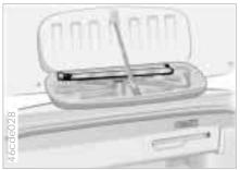
For easy access, the hazard warning triangle is stored in the onboard tool kit in the luggage compartment lid.
