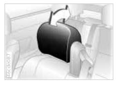
2 Tilt angleManually position the head restraint as
