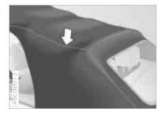
4 Position the rear convertible top bar vertically and hold it firmly
